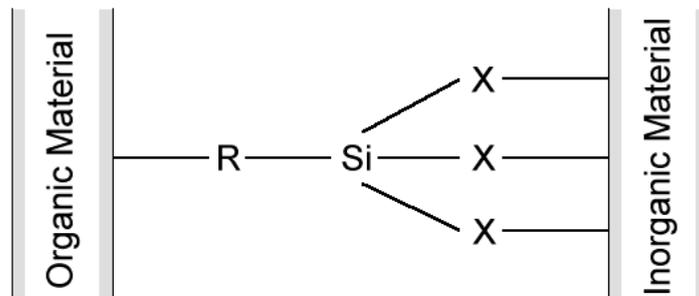
Silicon (Si) is the center of the silane molecule which contains an organic functional group (R) [ex: vinyl, amino, chloro, epoxy, mercapto, etc.], with a second functional group (X) [ex: methoxy, ethoxy, etc.]. The functional group (R) will attach to an organic resin while the functional group (X) attaches to an inorganic material or substrate to achieve a "coupling" effect.
